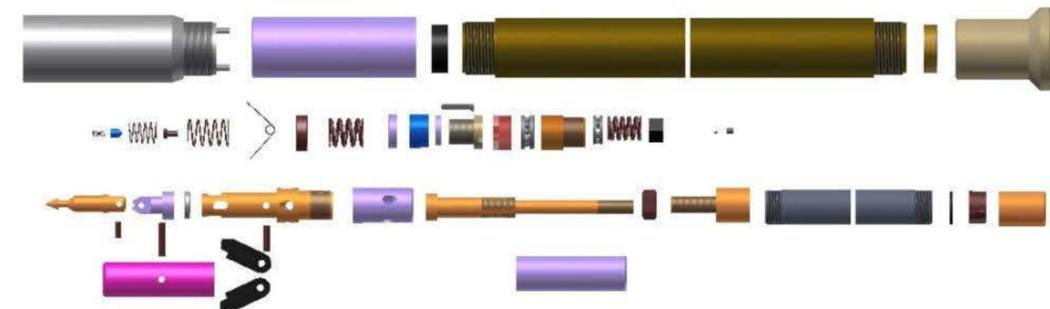
煤层气绳索取心钻具CBM (Coal Bed Methane) wire-line coring drill tools
